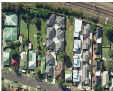
Figure 1 – Comparison of existing low density housing with Codes SEPP development standards. Loss of deep soil is evident with newer development that allows on-grade car parking with associated extensive hardstand and roof coverage with little to no deep soil areas remaining.
